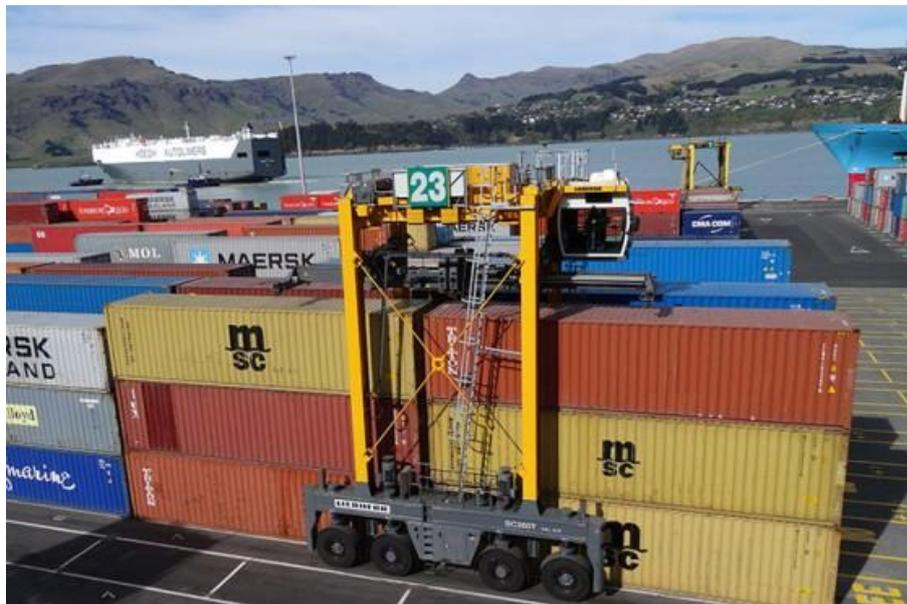
Image B1.1 – Example of a Straddle Carrier
