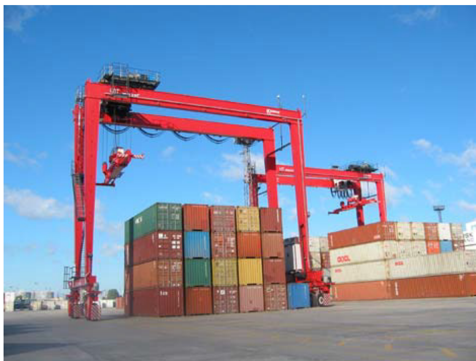
Figure 3.04 - Typical Rubber Tyred Gantry Crane
